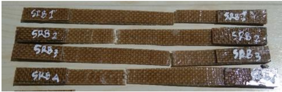
Fig. 6. Failure modes of RFRP under tensile test
