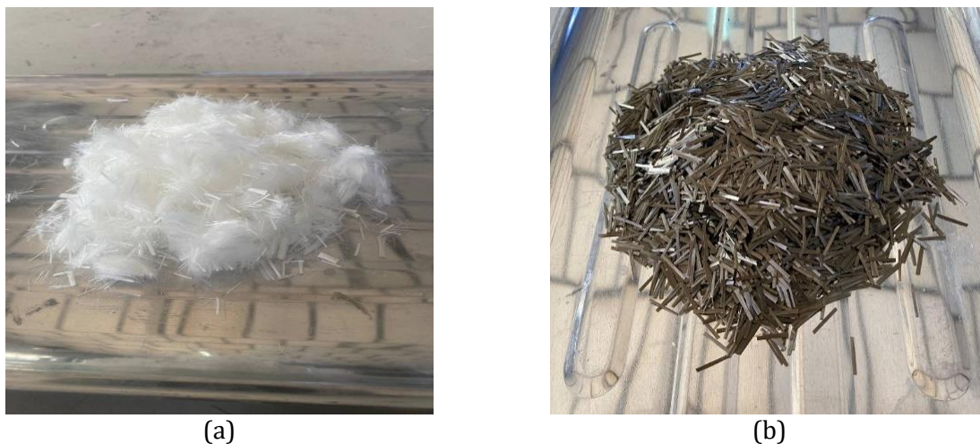
Fig. 1. (a) PVA fiber 6mm and (b) basalt fiber 12 mm
