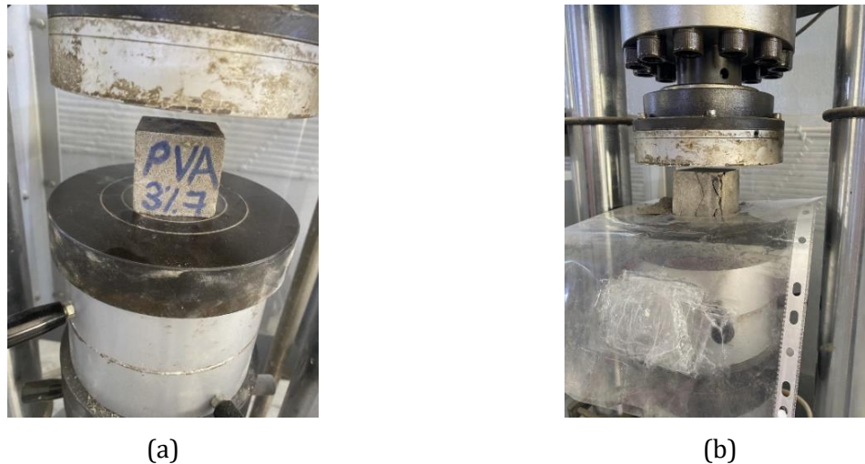
Fig. 4. (a) Compression cubic before failure and (b) the cubic after failure
