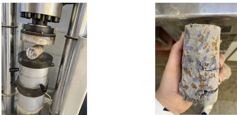
Fig. 14. The cylinder before and after failure
