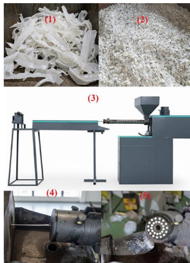
Fig. 4. Stages of recycling polypropylene waste into pellets or 3D-printing filaments
