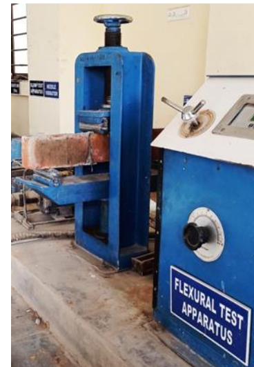
Fig. 7. Flexural strength test for masonry: (a) Schematic diagram and (b) test set-up
