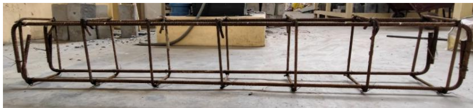
Fig. 4. Reinforcement configuration of tested beams shown in real and schematic forms A) RCSF0% B) RCSF1.0% C) Demonstrates actual reinforcement configuration
