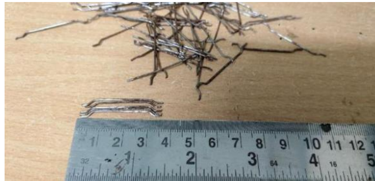
Fig. 2. Representative steel fiber materials utilized in the experimental program
