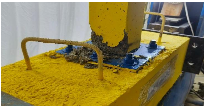
Fig. 24. Failure mode of (6 P10 A16 W1 -5) specimen
