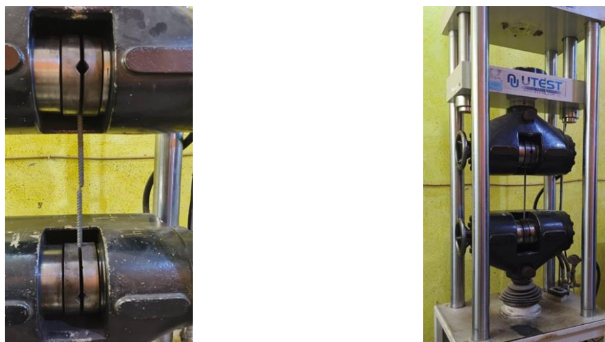
Fig. 6. Tensile testing machine for steel reinforcement
