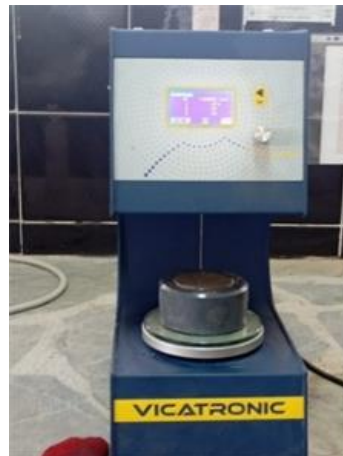
Fig. 6. Setting test using the Vicat method
