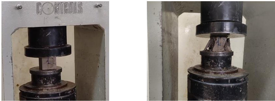
Fig 16. Compressive strength test of mortar cubes
