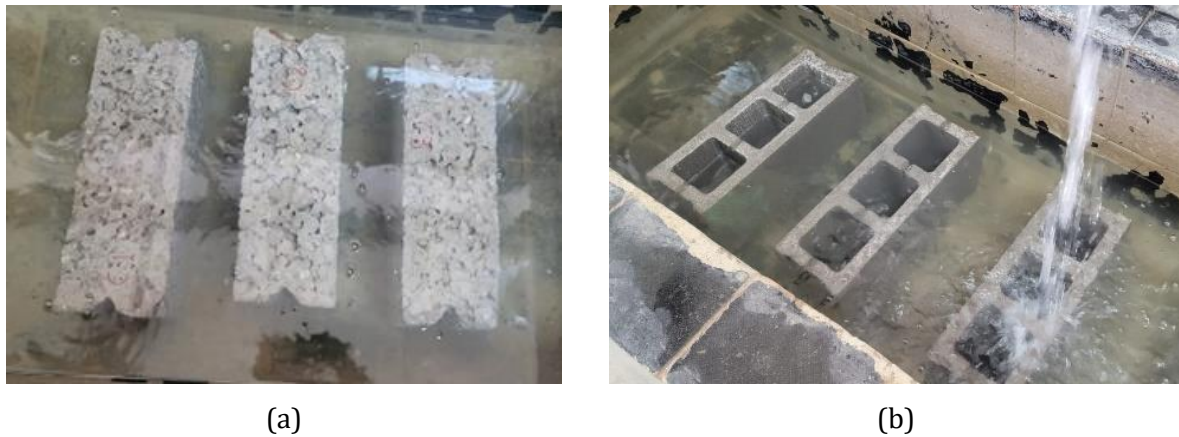
Fig. 10. Water Absorption Test on Blocks (a) Caramelo block and (b) Pressed block
