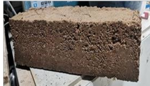
(b) Reinforced soil beam
