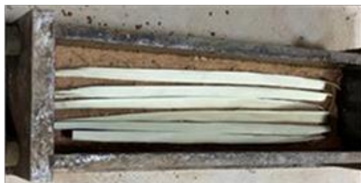
(a) Strips laid on top of a second compacted soil layer
