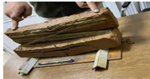
(b) Reinforced soil beam at failure prepared for testing
