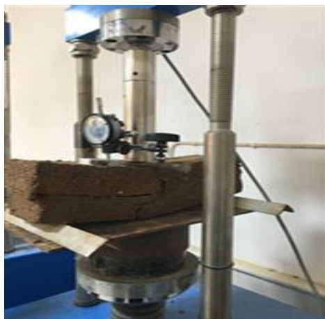
(a) Soil beam at failure case during applied stress
