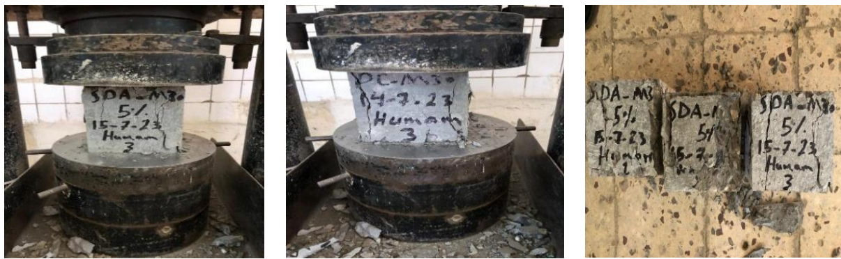
(a) Specimen identification (b) Specimen at failure (c) Failure mode
