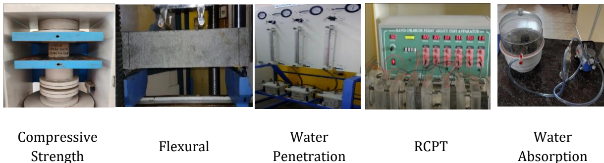
Fig. 12. Tests conducted on the strength and durability properties of SCC mixes
