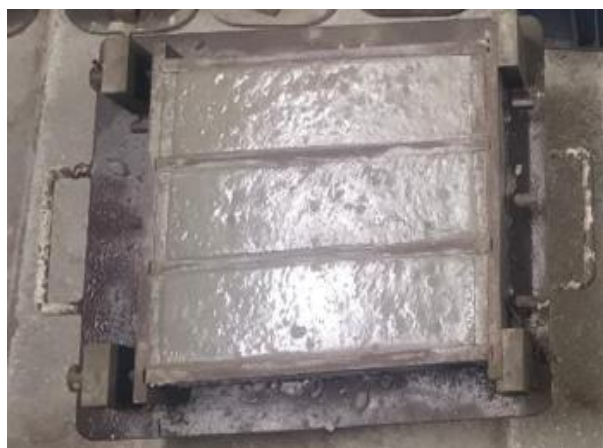
(a) Specimens cast in the mould
