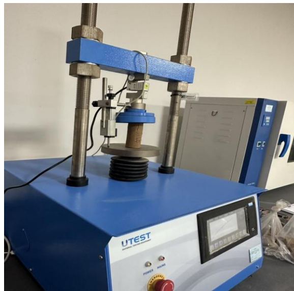
Fig. 5. Test setup for unconfined compressive strength
