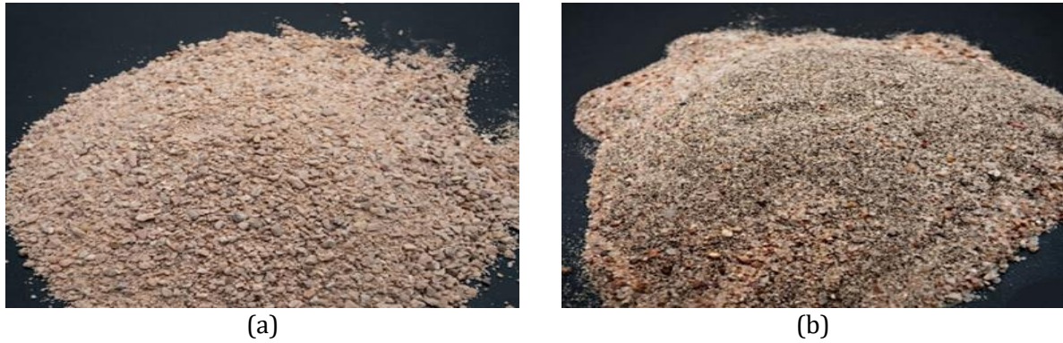
Fig. 1. Illustrative types of fine aggregates used in this study (a)Crushed aggregate, (b) River aggregate
