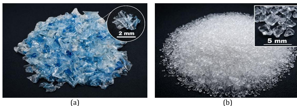
Fig. 2. Illustrative types of waste are used in the study (a): Crushed waste glass (WG) and (b): Waste polyethylene terephthalate (WPET)
