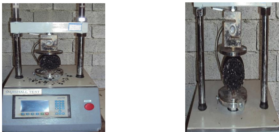
Fig. 3. Illustrative indirect tensile strength test
