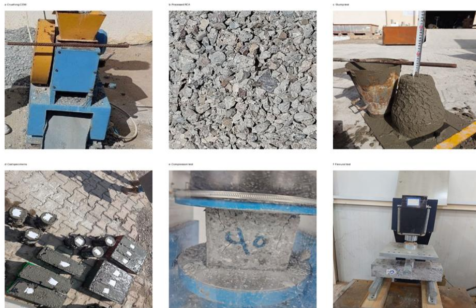
Figure 1. Experimental program: (a) crushing concrete debris; (b) processed RCA; (c) slump measurement; (d) cast specimens; (e) compression testing; and (f) flexural testing. Photographs supplied by the author
