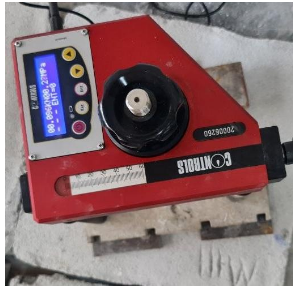
Figure 3. Pull-off strength test
