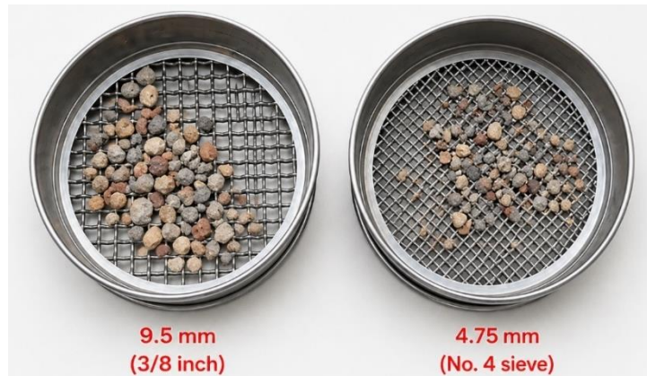
Fig. 2. Selected pumice fraction used in the study (passing 9.5 mm and retained on 4.75 mm sieve)
