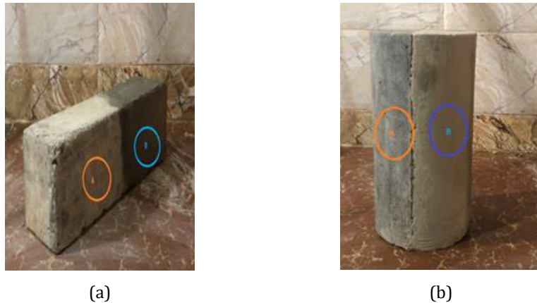
Fig. 1. The Composite specimens (a) old concrete, (b) repair
