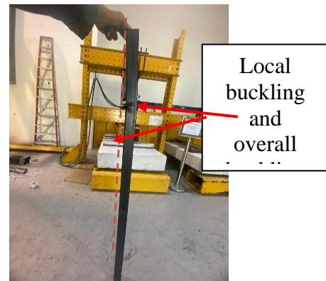
Fig. 9. Failure modes for a single SHS column of S3-H2-SHS
