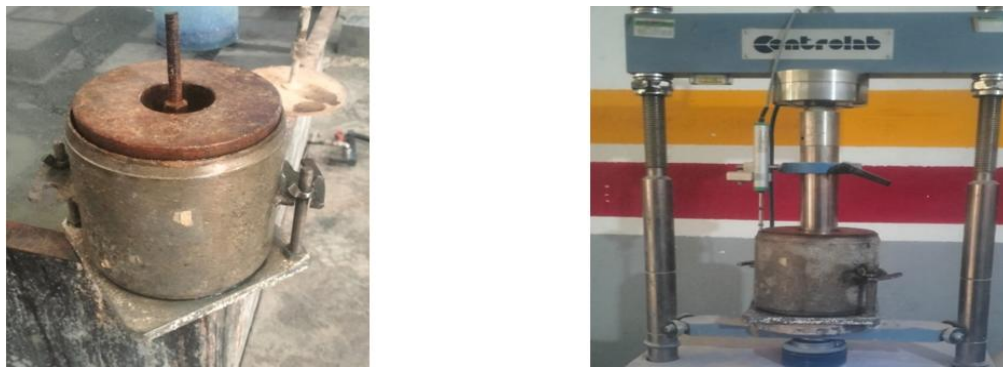
Fig. 4. CBR test for compacted mixtures
