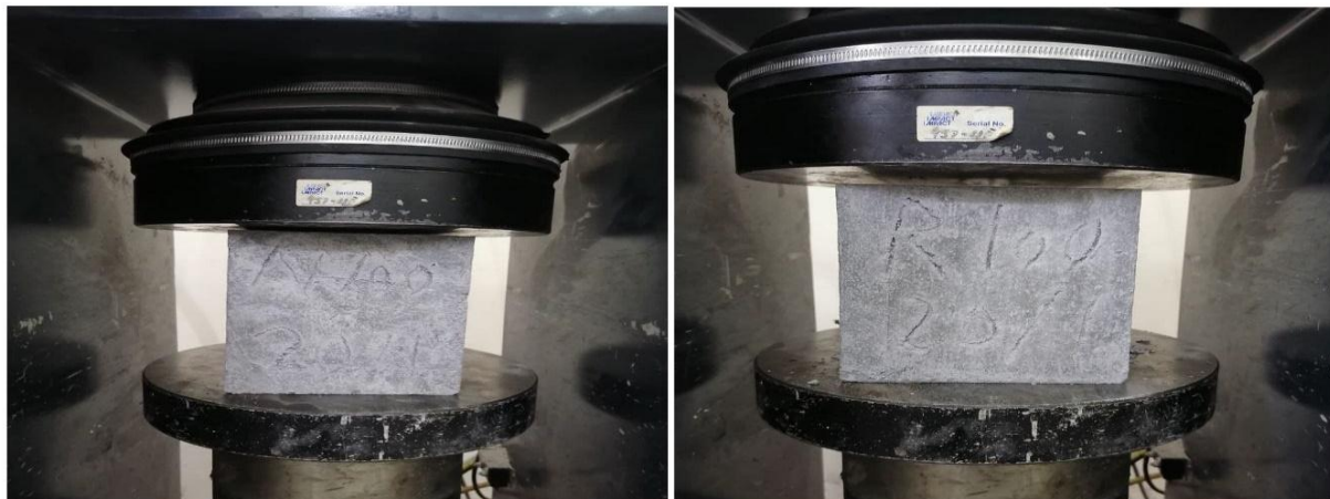
Fig. 4. Cube compression test of hardened concrete
