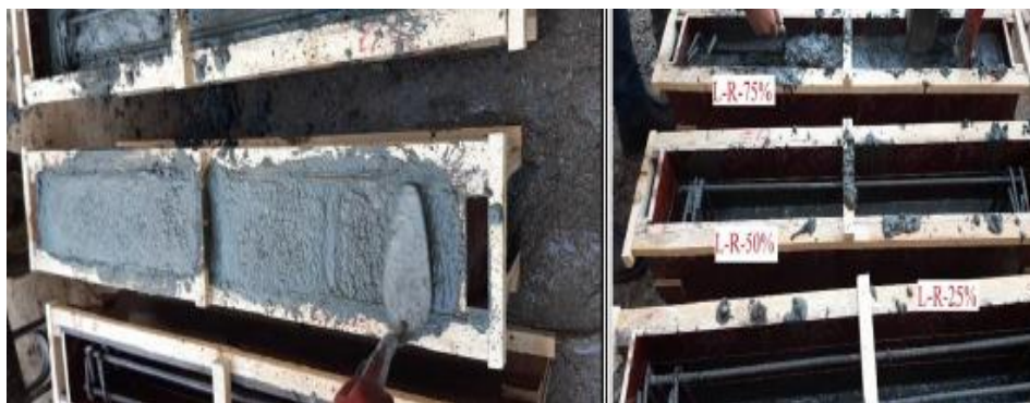
Fig. 10. Casting with R-100% at layers
