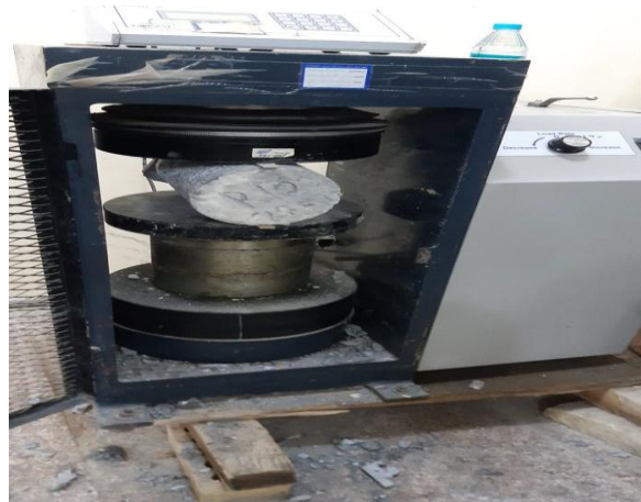
Fig. 6. Splitting tensile strength test of hardened concrete
