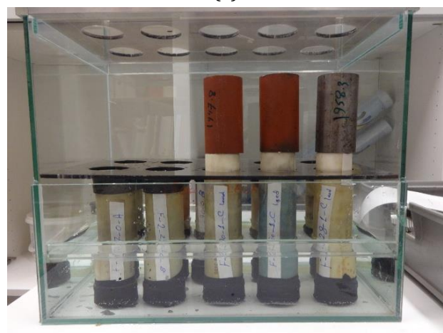
Fig. 2. Shown two different curing conditions (a) Schematic sketch and (b) Two specimens sets cured under different conditions
