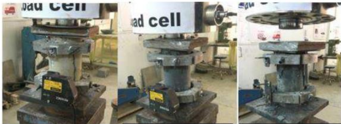
Fig. 12. Progressive compressive failure observed during cylinder testing
