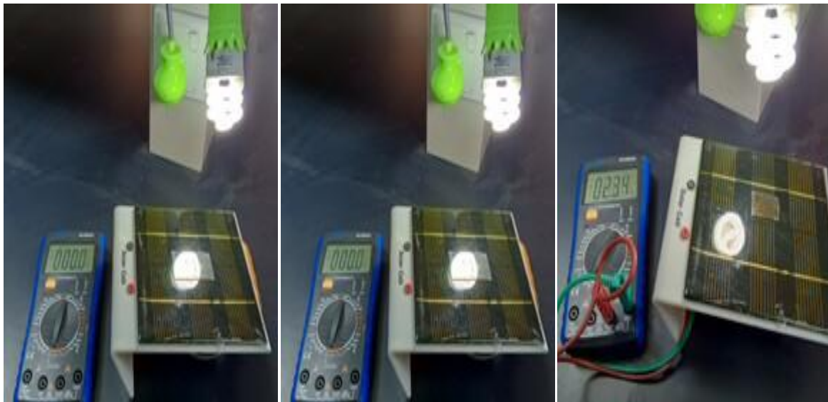
Fig. 6. Output voltage increase of a solar cell due to the effect of nanophotonics thin films and light
