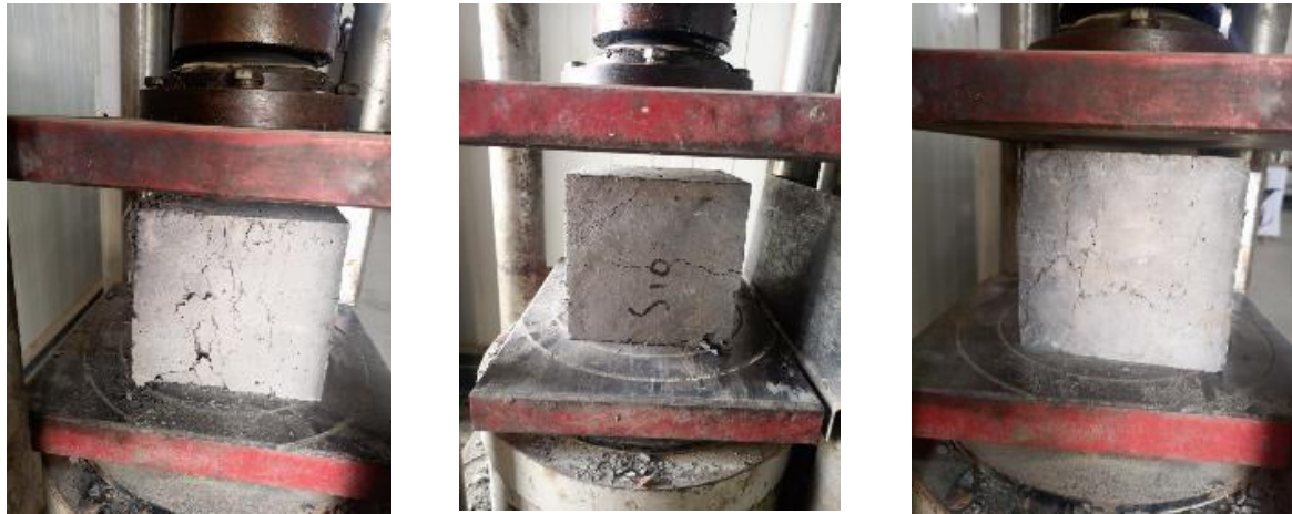
Fig. 13. Compressive strength failure for some specimens
