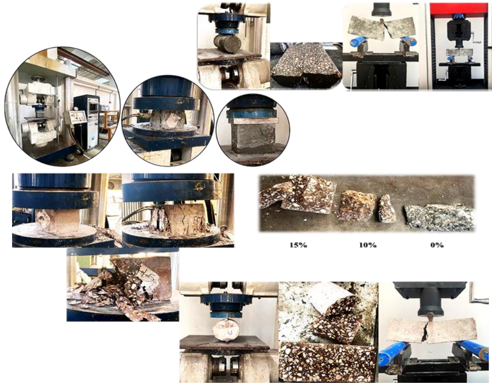
Fig. 6. Mechanical strengths tests of normal and modified-concrete mixes
