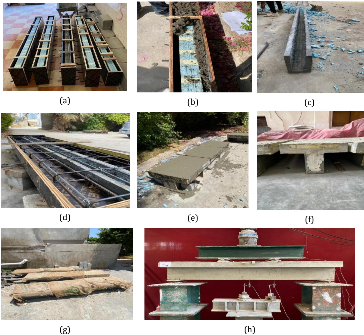
Fig. 10. Flow chart of the composite beam fabrication process: (a) preparing formwork; (b) casting UHPFRC plates; (c) demolishing formwork; (d) setting up steel reinforcement; (e) casting concrete core and flange; (f) demolishing flange formwork; (g) curing; (h) testing
