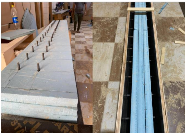
Fig. 8. Prepared inner and external formwork for S4-SC beam
