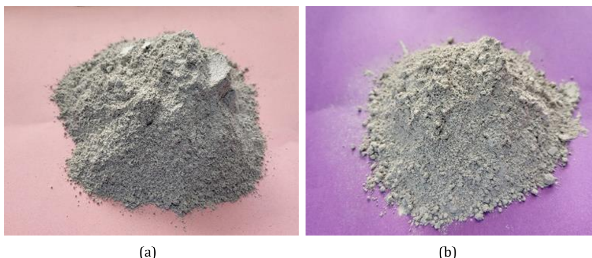
Fig. 3. (a) Concrete Demolition Powders, and (b) Concrete Sample Scraps Powders
