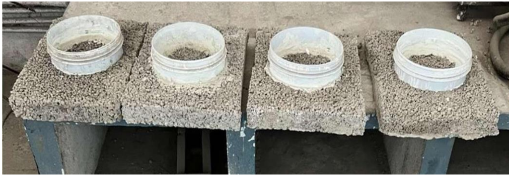
Fig. 2. Rings sealed to the surface of slab specimen as per ASTM C1701 (2)
