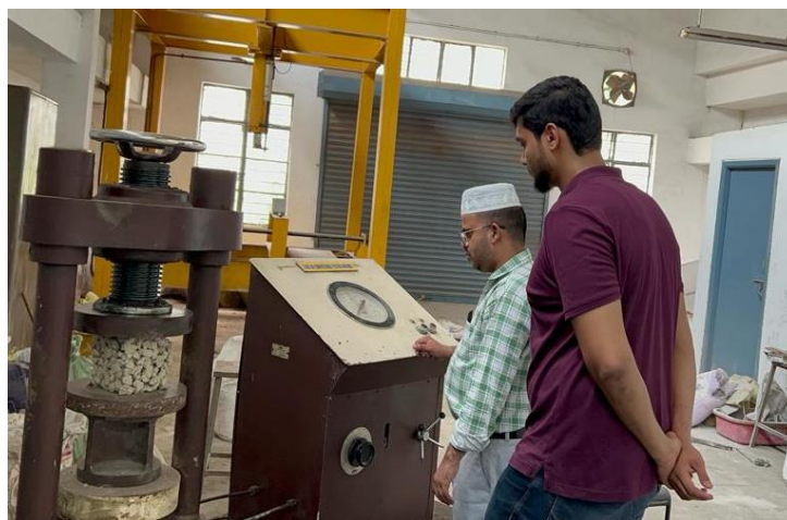
Fig. 4. Compressive test on Cube Specimens
