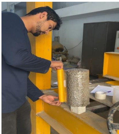
Fig. 6. Using shrink wrap to wrap specimen for infiltration test
