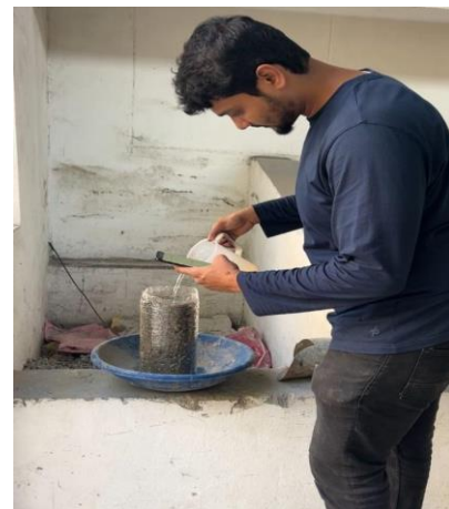
Fig. 7. Infiltration test of Pervious concrete cylinder
