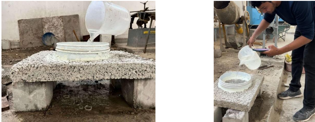
Fig. 5. Infiltration test of Pervious concrete slab
