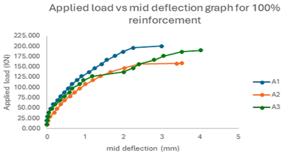
Fig. 11. Applied load vs mid-deflection for 100% reinforcement
