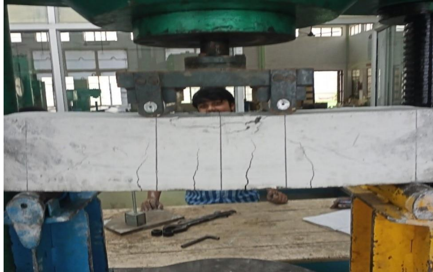
Fig. 9. Specimen crack for 70% reinforcement
