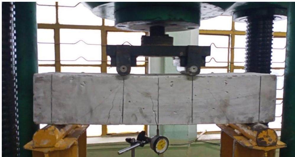
Fig. 8. Specimen crack for 100% reinforcement
