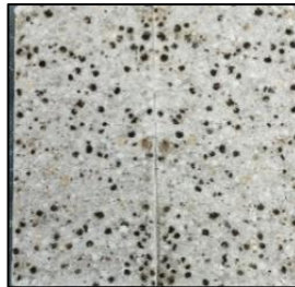
Fig.12. Fractured lightweight concrete specimen after split tensile test
