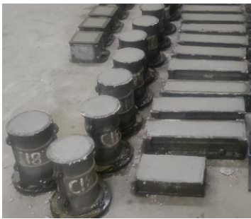
Fig. 6. Concrete cubes, cylinders, and beams in molds
