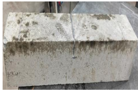
Fig. 7. Notched beam sample
