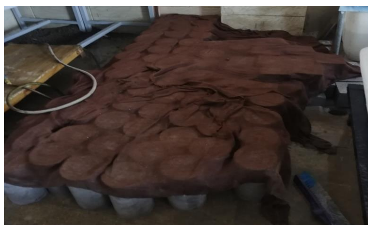
Fig. 8. Processing samples with a wet cover in the concrete laboratory
