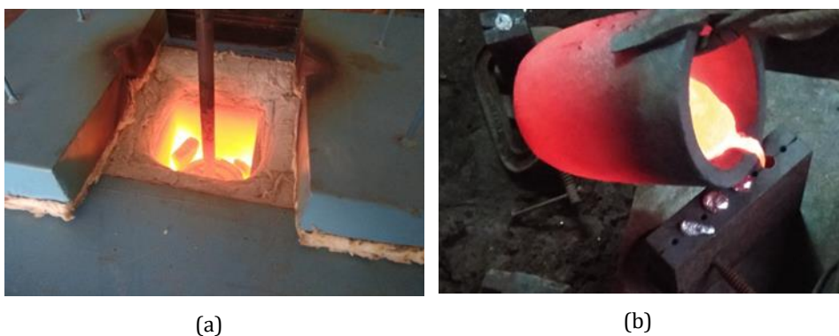
Fig. 2. Showing the (a) Molten metal in electric furnace (b) Cast iron die used to prepare samples
