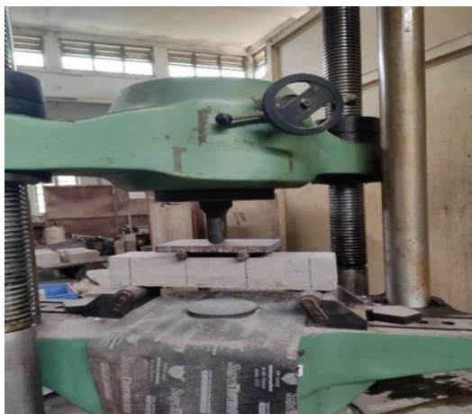
Fig. 8. Flexural strength test using 100T UTM
