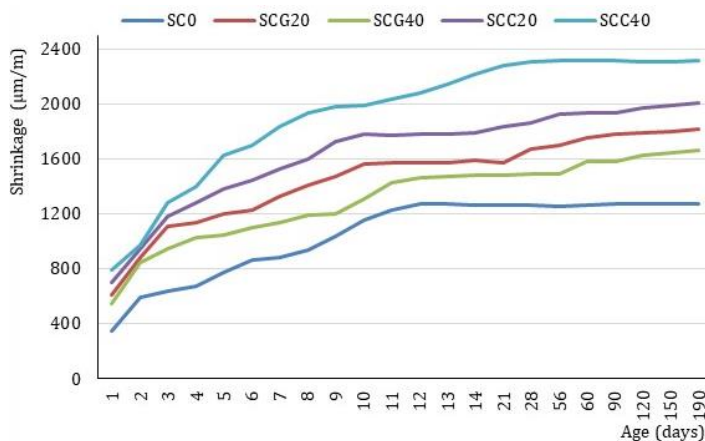
Fig. 14. Influence of substitution rate and type of sand on shrinkage
