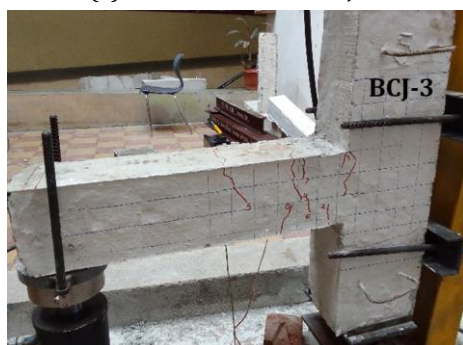
(a) Crack Patterns of BCJ-3
