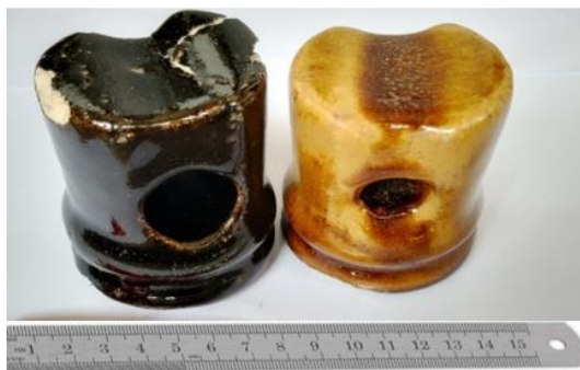
Fig. 2. The produced porcelain insulators at different levels of glazing
