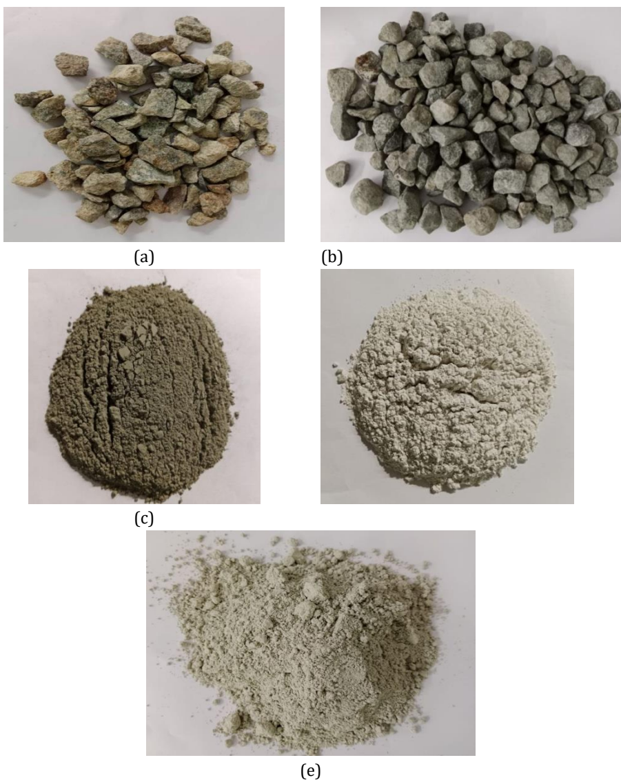
Fig. 2. Images of the materials used in the current study (a) recycled aggregate, (b) natural aggregate, (c) cement, (d) ggbs and (e) crete
