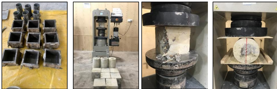
Fig. 4. Photograph of compressive strength testing and splitting tensile strength
