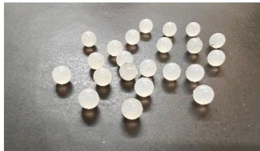
Fig. 2. Compression molding process of silicone rubber particle production and silicone rubber particles
