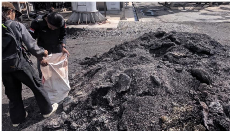
Fig. 3. Slag from burning palm shell ash
