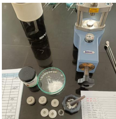
Fig. 6. Sample preparation for FTIR testing
