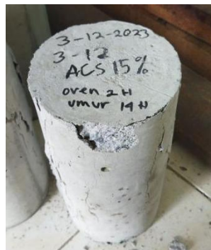
Fig. 7. Sample concrete after compression test
