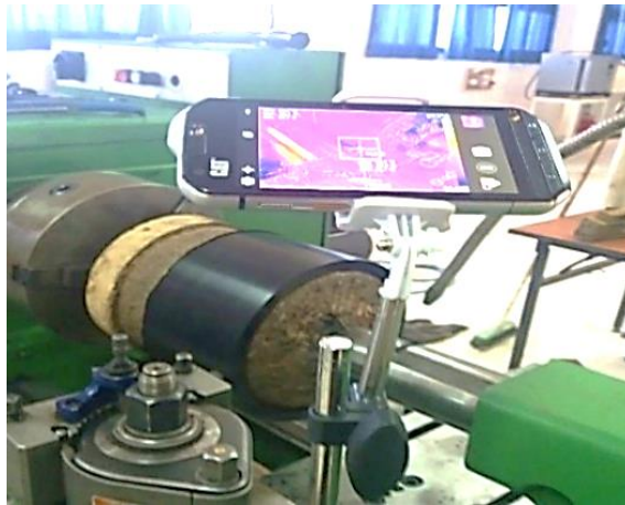
Fig. 2. Temperature measurement set-up using CAT S60 smartphone [13]
