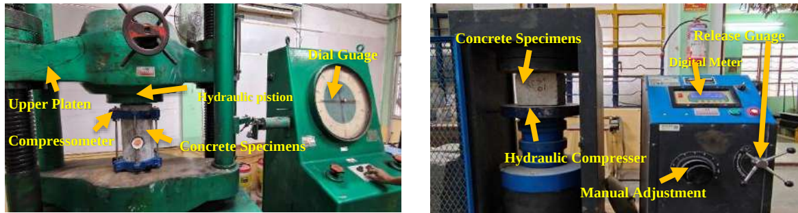
Fig. 3. Experimental test setup of compression testing machine for concrete specimens
