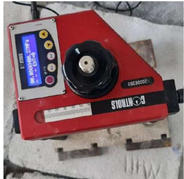
Figure 3. Pull-off strength test
