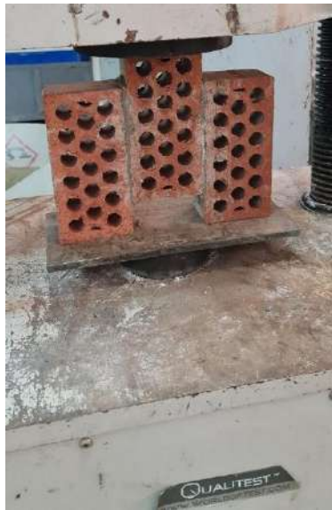
Figure 2. Shear strength test (Triplet test)
