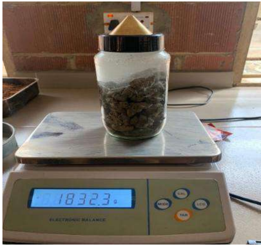
Fig. 3. Particle Density Apparatus – Pycnometer Technique
