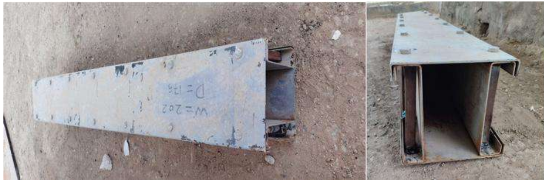
Fig. 10. Failure Mode of Beam BH1.15
