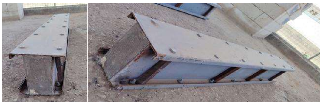
Fig. 23. Failure mode of beam BC0.85
