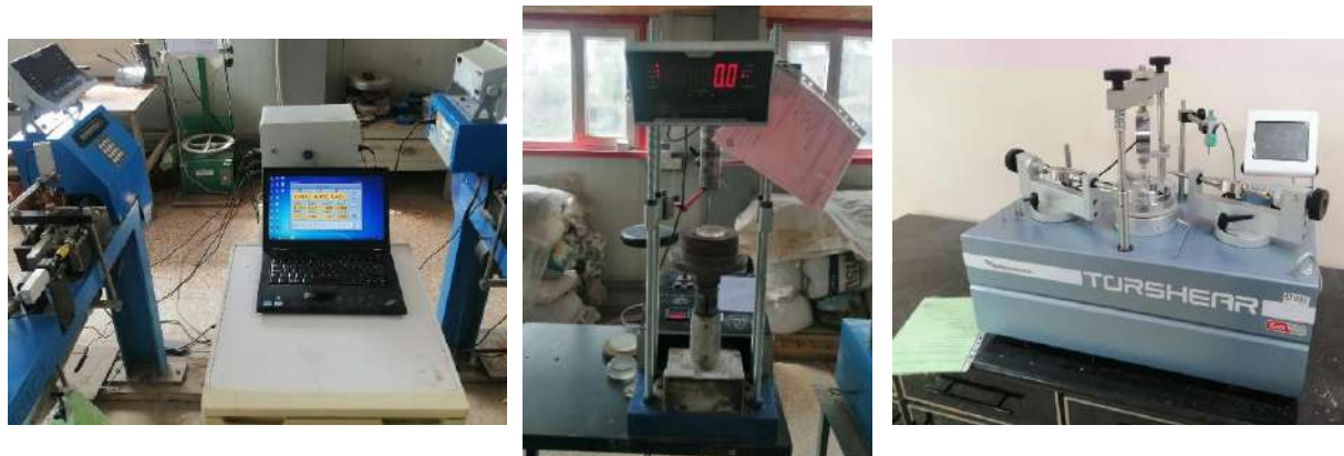
Fig. 2. Equipment used in the study, left: direct shear, middle: unconfined compression, right: residual shear.
