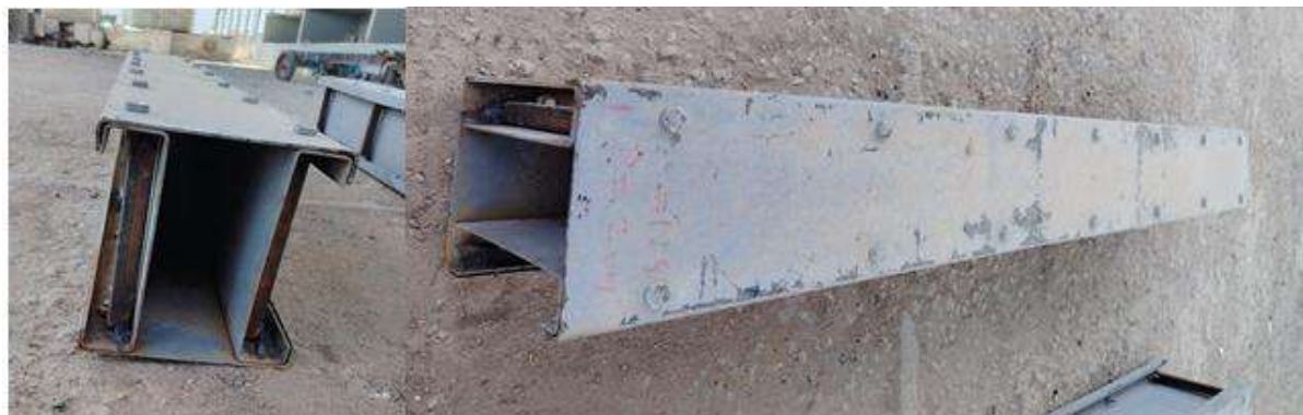
Fig 12. Failure Mode of Beam BH0.85
