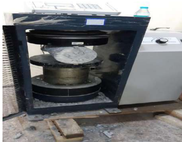
Fig. 6. Splitting tensile strength test of hardened concrete
