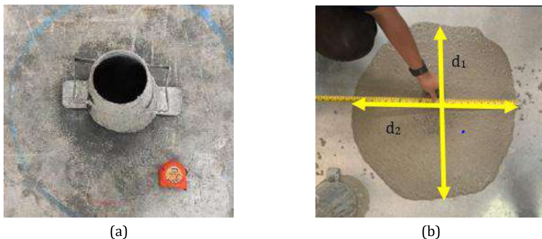
Fig. 6. Equipment and measurement procedure for the slump flow and T500 test: (a) Experiment set-up; (b) diameter measurement ( d_1 and d_2 )
