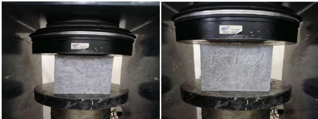
Fig. 4. Cube compression test of hardened concrete
