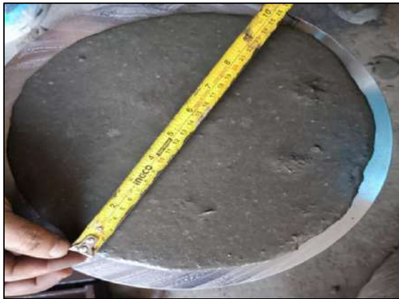
Fig.4. Flow table test of RPC mixtures
