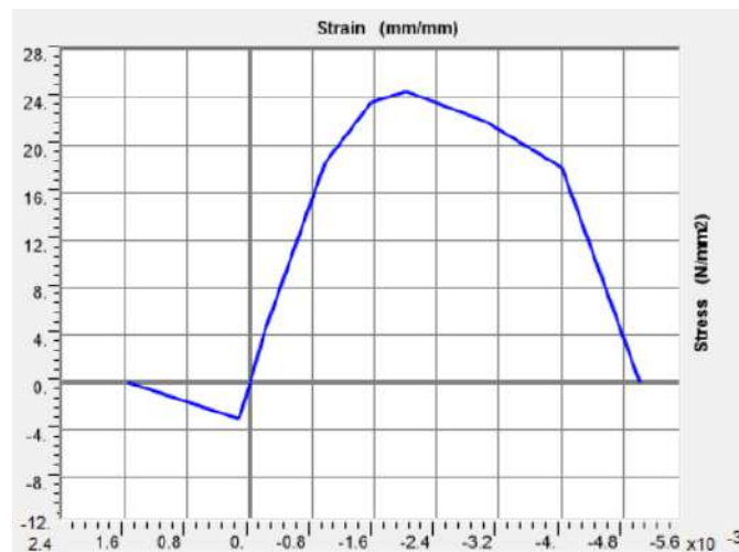
Fig. 10. Constitutive model of the nonlinear behavior of concrete in analyses (1 Mpa=1N/mm 2 )
