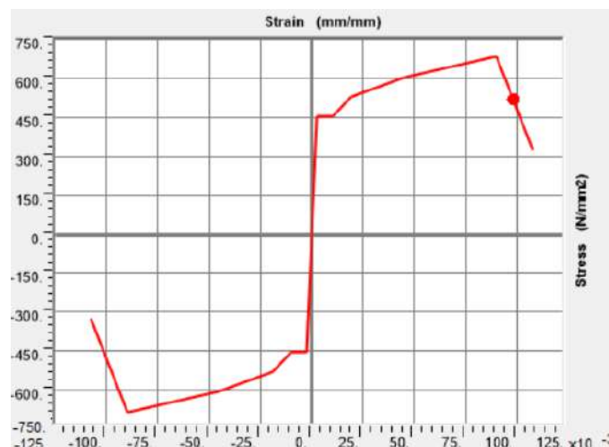
Fig. 11. Constitutive model of the nonlinear behavior of steel in analyses (1 Mpa=1N/mm 2 )
