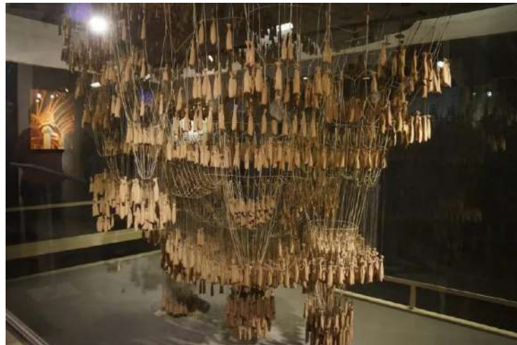
Fig. 1. The idea behind La Sagrada Familia: Gaudí's hanging chain model. Available from: https://parametric-architecture.com/la-sagrada-familia-gaudis-chain-model/
