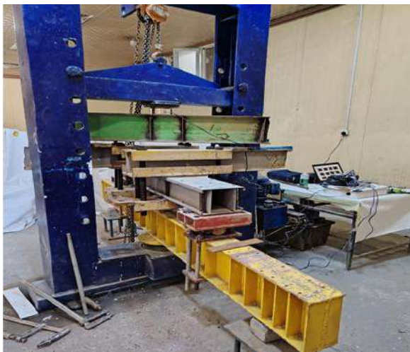
Fig. 6. Member under Torsional load
