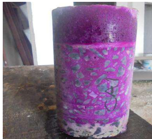
Fig. 10. Carbonation for Phase 1 Mix (0% RAC-Control-CA1) concrete sample
