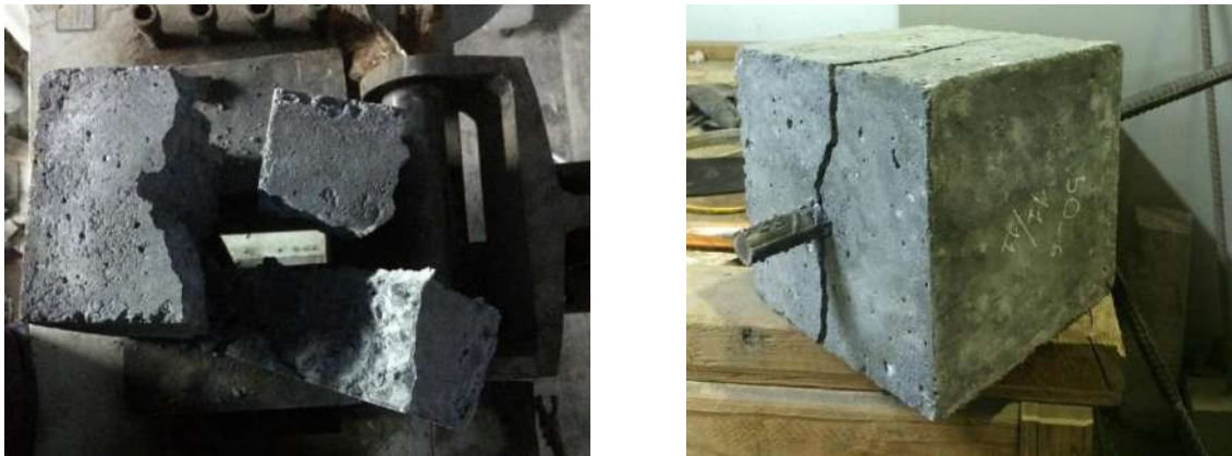
Fig. 5. Failure modes observed after testing
