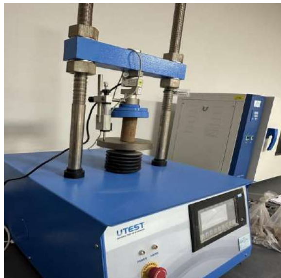
Fig. 5. Test setup for unconfined compressive strength
