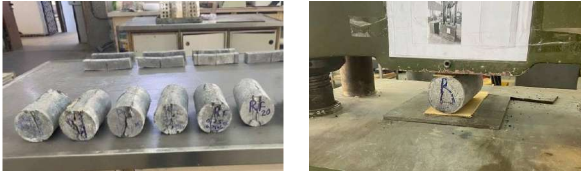
Fig. 6. Testing and failure of the specimens
