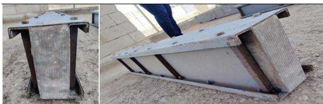
Fig. 24. Failure mode of beam BC0.7
