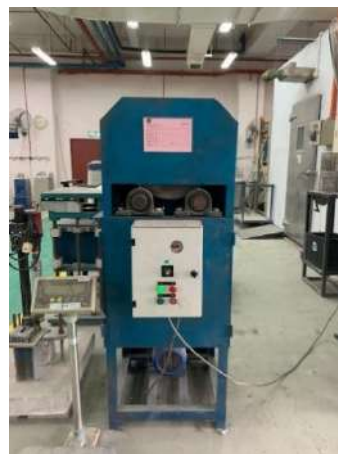
Fig. 2. Mechanical grinder used for processing eggshells into fine powder (ESP)
