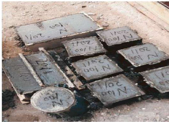
Fig. 3. Specimens of hardened concrete
