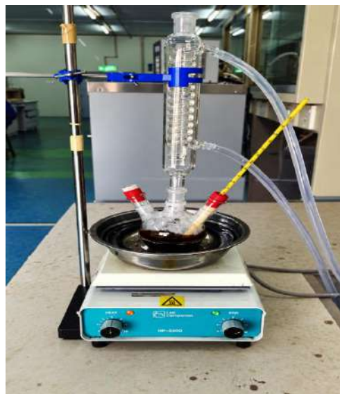
Fig. 2. The transesterification experimental setup
