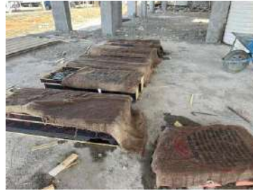
(e) Specimens retained under wet burlap after casting
