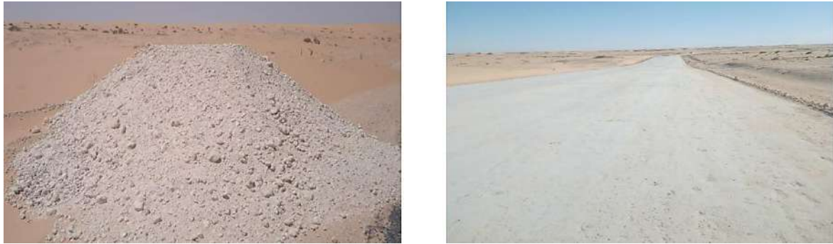
Fig. 1. Gypseous-calcareous soil before and after compaction
