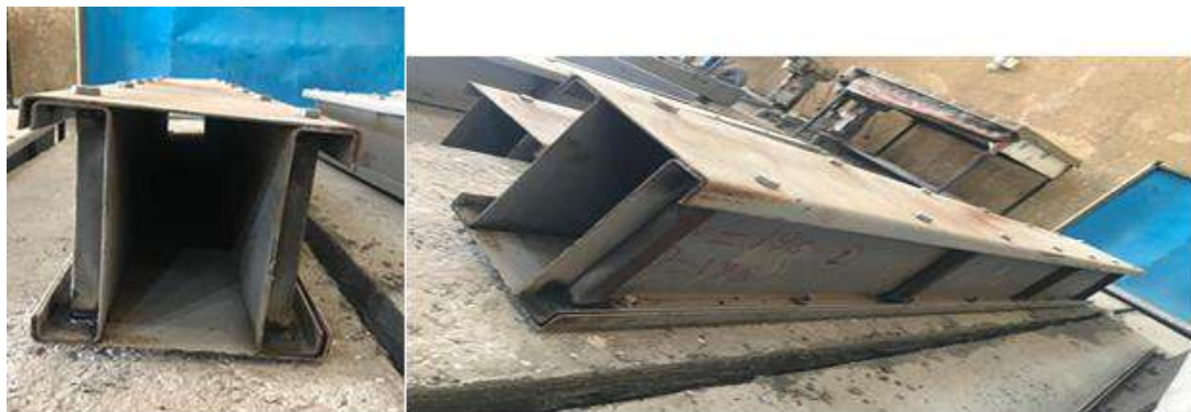
Fig. 11. Failure Mode of Beam BH1
