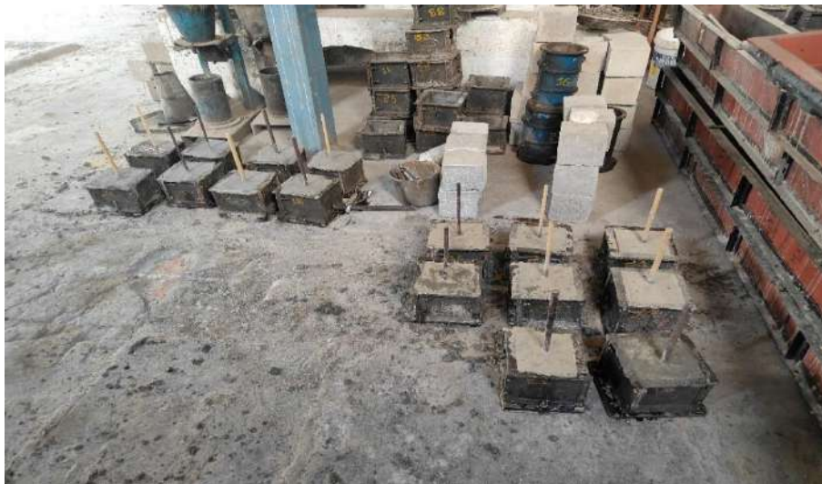
Fig. 2. GFRP bars and steel bar pullout specimens
