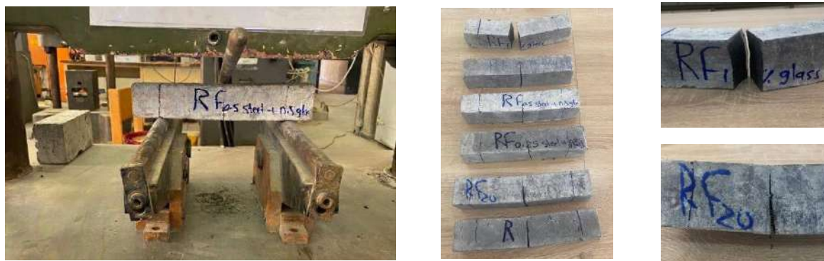
Fig 5. Testing and failure of the specimens
