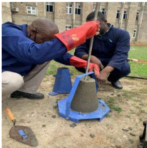
Fig. 7. Experiment on the workability of concrete specimen
