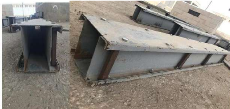
Fig. 9. Failure Mode of Beam BH1.3
