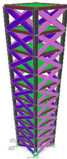
Fig. 3. Finite element model of the infill wall
