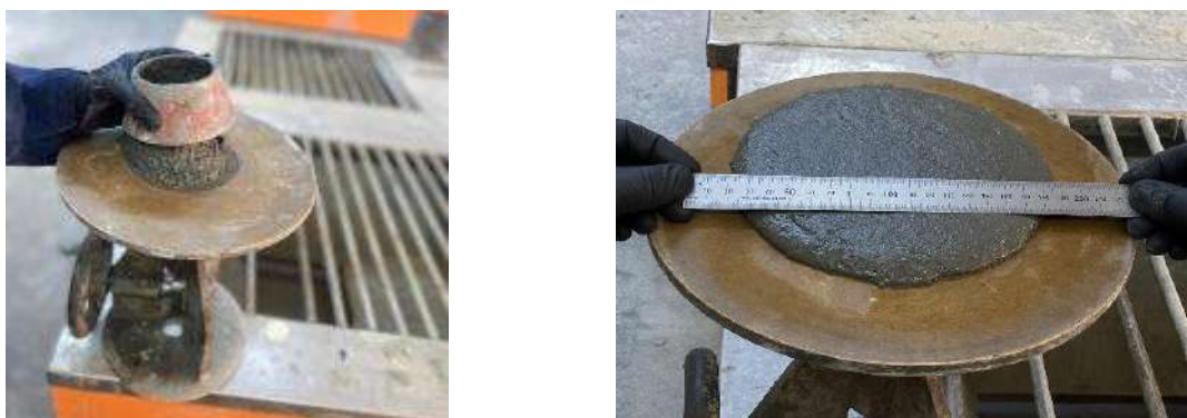
Fig. 2. Flow table test procedure
