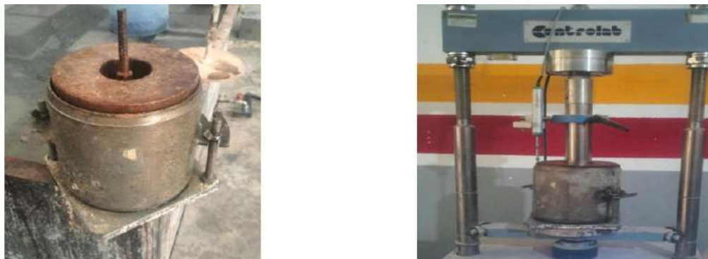
Fig. 4. CBR test for compacted mixtures
