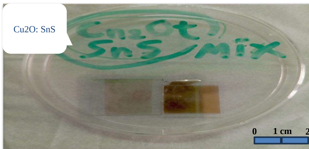
Fig. 3. Cuprous oxide Cu 2 O: SnS nanophotonics glass thin film prepared
