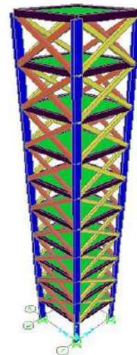
Fig. 4. Finite element model of the infill wall with a soft story
