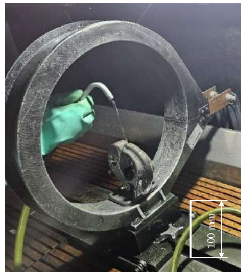
Fig. 2. Aircraft tow hook sample washing with magnetic particle testing solution
