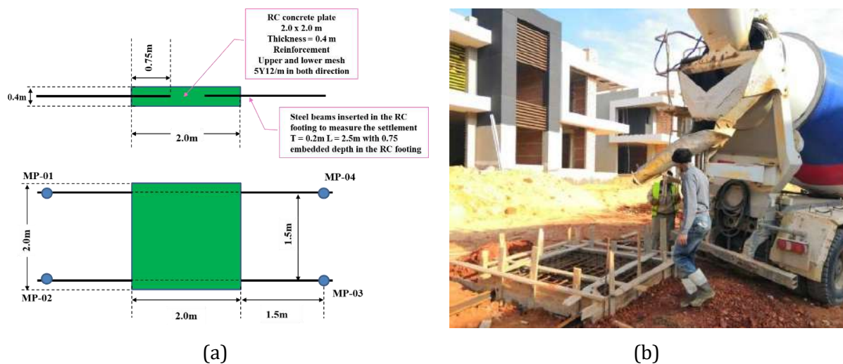
Fig. 12. Construction of RC footing (a) Schematic (b) Photograph
