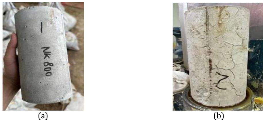
Fig. 15. Physical condition of normal concrete specimens before and after exposure to 800°C: (a) before burning, bright gray in color; (b) after burning, showing a yellowish-gray color, longer cracks, and increased spalling
