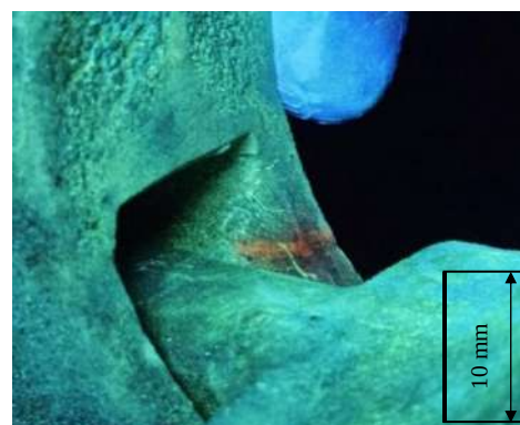
Fig. 9. Observed discontinuities after liquid penetrant testing
