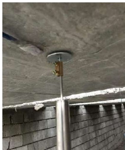
Fig. 4. Dynamic LVDT and accelerometer
