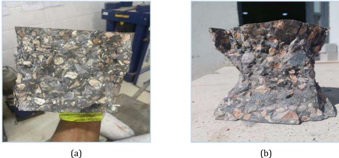
Fig. 9. Form of rupture of specimens without and with water-repellent
