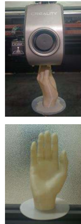
Fig. 14. 3D printed model of recycled polypropylene
