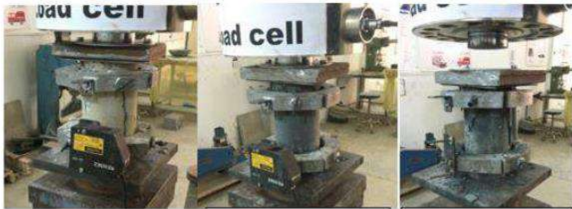
Fig. 12. Progressive compressive failure observed during cylinder testing
