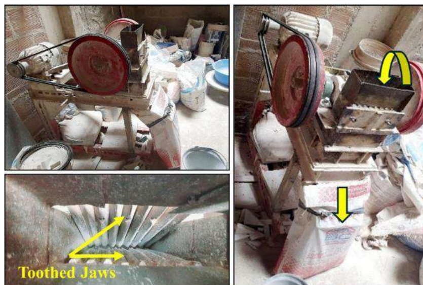
Fig. 1. Toothed jaw crusher used for crushing aggregates
