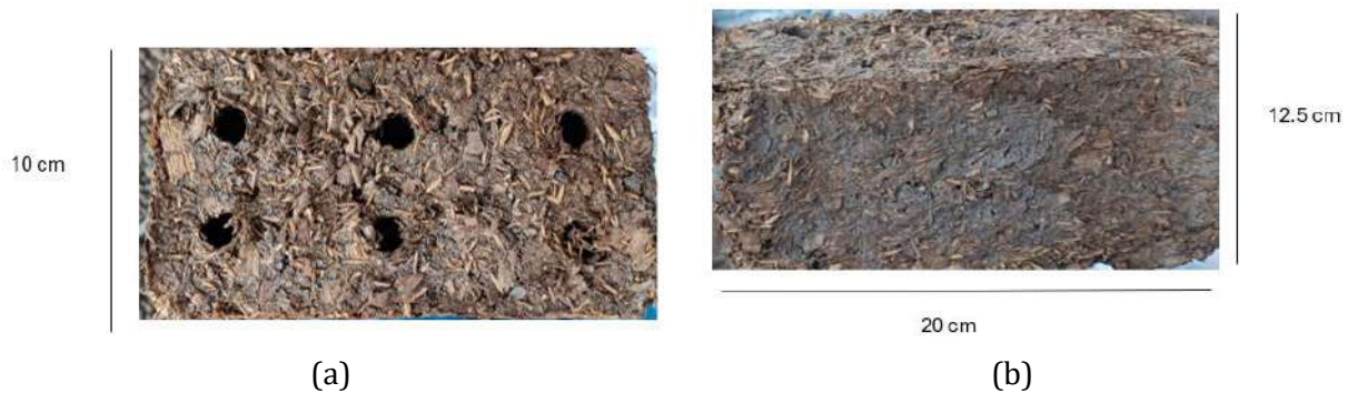
Fig. 1. Geometry and appearance of the produced briquette: (a) top view (left) showing surface perforation holes; (b) side view (right). Nominal dimensions are 20 cm × 10 cm × 12.5 cm (length × width × height)
