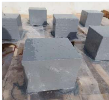
Fig. 5. Application of epoxy
