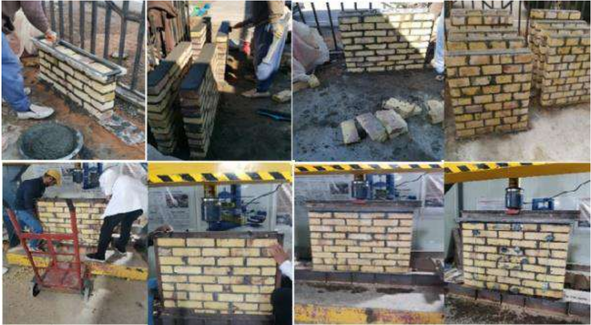
Fig. 4. Construction and setup of walls to test
