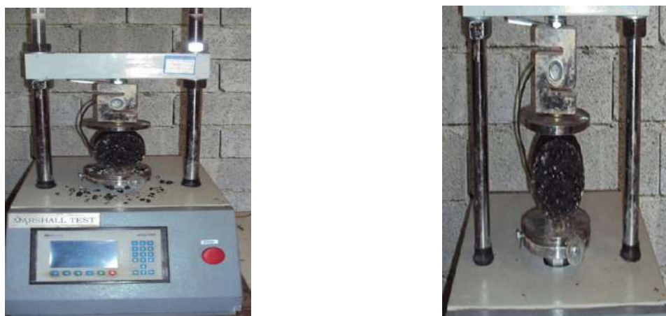
Fig. 3. Illustrative indirect tensile strength test
