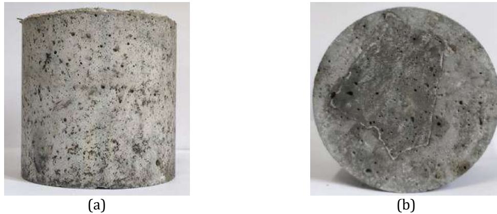
Fig. 2. Brazilian disc specimen (BD) (a) Front and (b) Vertical
