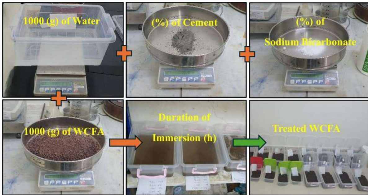
Fig. 3. Photos illustrating WCFA treatment process
