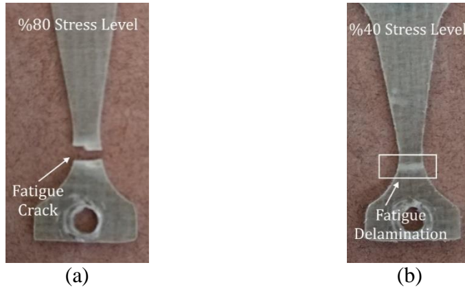
Fig. 8 Fatigue damage of glass/epoxy composite (a) crack and (b) delamination
