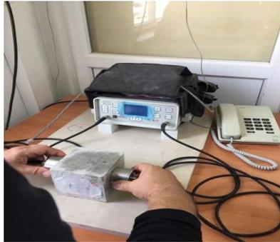
Fig. 3 Ultrasonic measuring instrument
