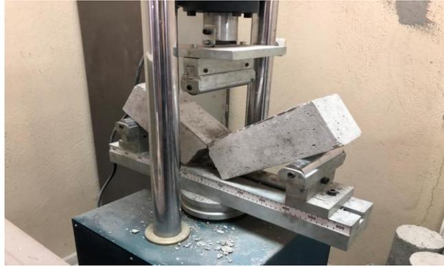
Fig. 5 Three-point flexural test
