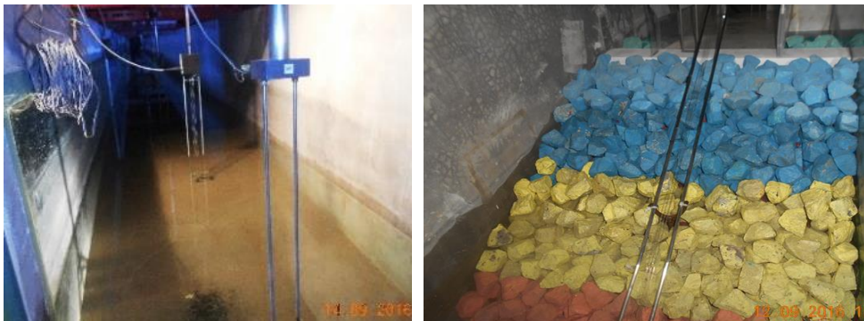
Fig. 4 . Measuring equipment. Left: wave gauges to measure free surface elevation; right: run-up wave gauge
