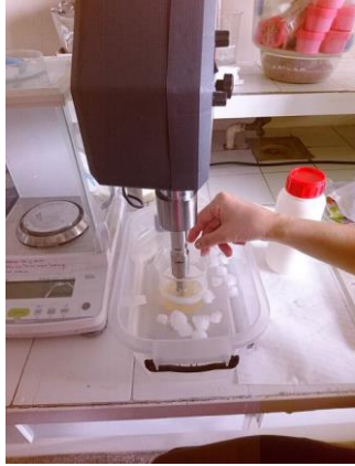
Fig. 1 Ultrasonic homogenizer for dispersion silica aerogel.
