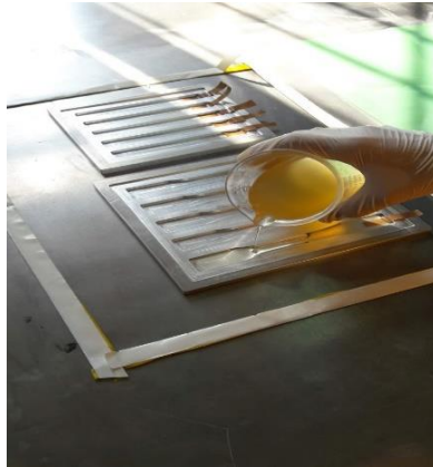
Fig. 2 Pouring mixture into aluminum mold.
