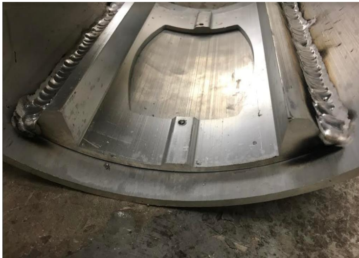
Fig. 3 Welded insert plate
