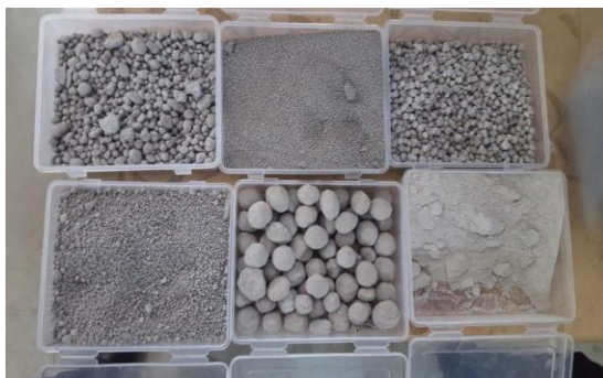
Fig. 1 Different Sizes of Light Weight Geopolymer Fly ash Sand (LWGFAS)
