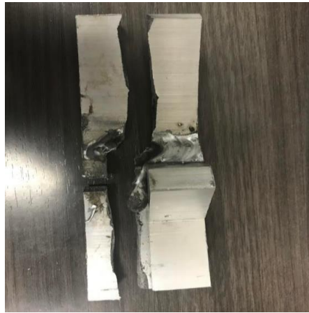
Fig. 10 Weld failure location
