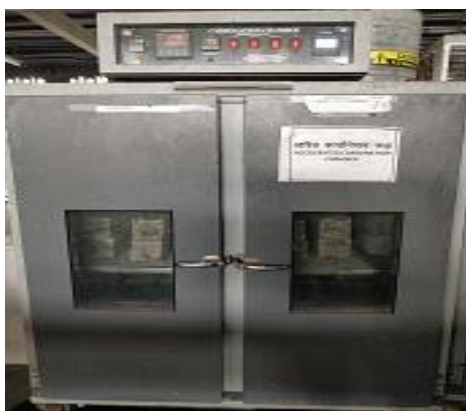
Fig. 6. Carbonation Chamber for Accelerated Carbonation Test
