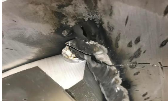
Fig. 9 Crack in weld
