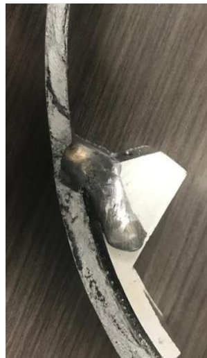
Fig. 11 Failure of pole sample
