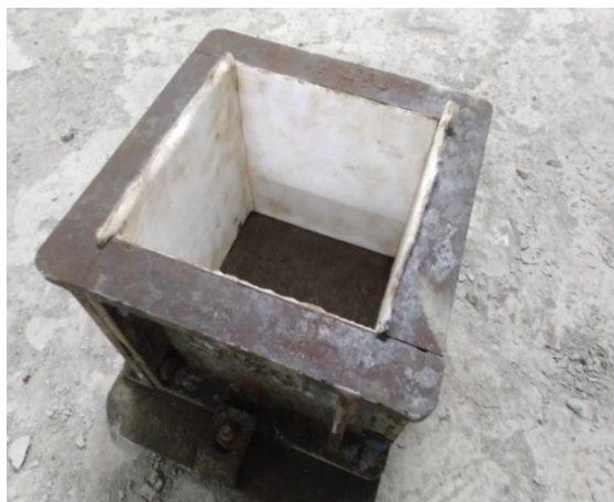
Fig. 2 Steel Mould with CPF Liner Pasted Inside
