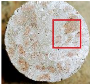
Fig. 9 Cross section of a hardened concrete at 800°C.
