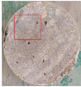
Fig. 8 Cross section of a hardened concrete at 400°C.
