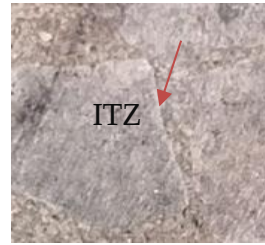
Fig. 8 Cross section of a hardened concrete at 400°C.
