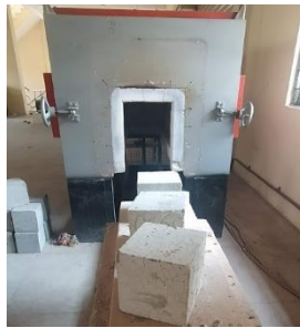
Fig. 3 Electric bogie for heating specimens
