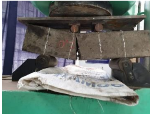
Fig. 3 Failure of specimens
