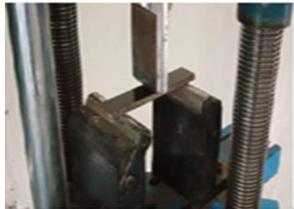
Fig. 6. Three-point bend testing set up for sandwich pane
