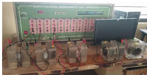
Fig. 4 Rapid chloride permeability test apparatus
