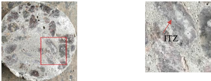
Fig. 7 Cross section of a hardened concrete at room temperature.
