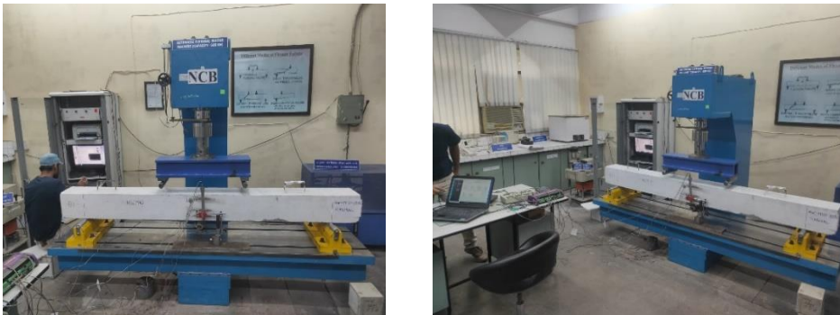
Fig. 3 (a) Beam in 4 point bend test and (b) Test Setup
