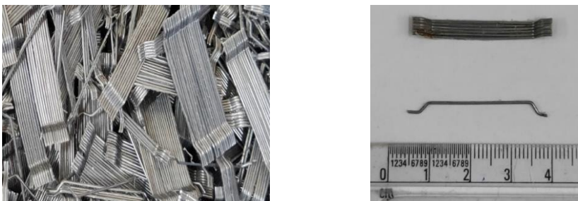
Fig. 2 Trough and hooked end shaped steel fibers
