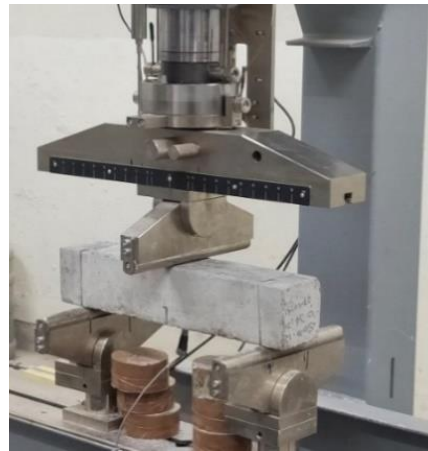
Fig. 4 Test set up for flexural strength
