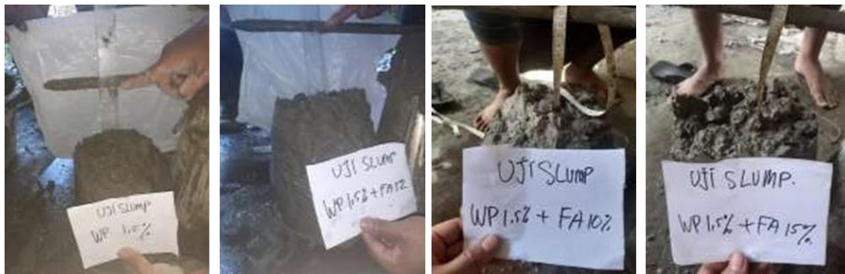
Fig. 3. Slump Abrams Test Measurement on BW, BWF1, BWF2, and BWF3
