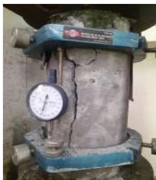
Fig. 7. The setting for testing modulus of elasticity
