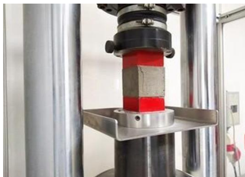
Fig. 3. Compression test setup of cube specimen
