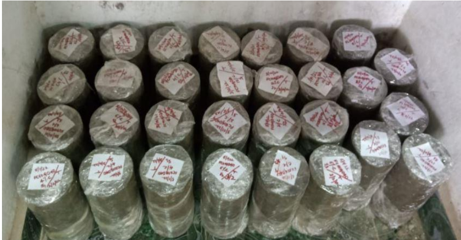
Fig.3 Cylindrical test specimens wrapped in polyethylene sheet
