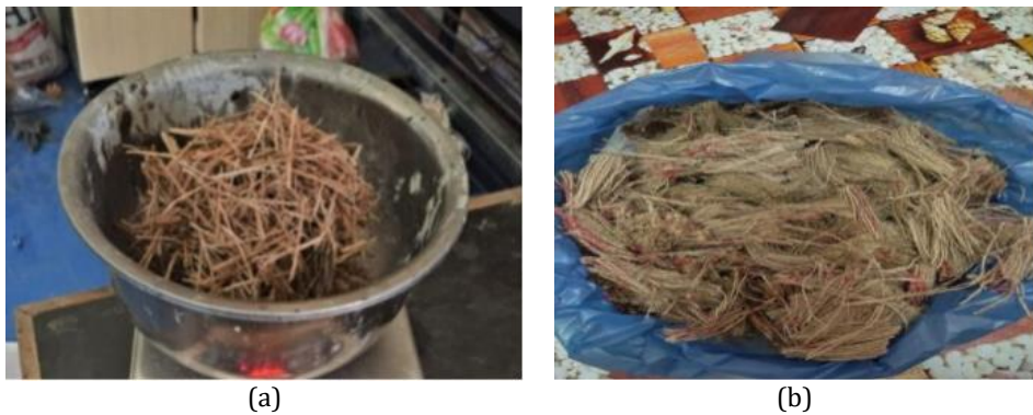
Fig. 3 Micro Reinforcement Bamboo (a) and Hemp (b)
