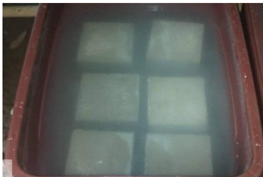
Fig. 4 Concrete cube samples cured in seawater in a controlled area
