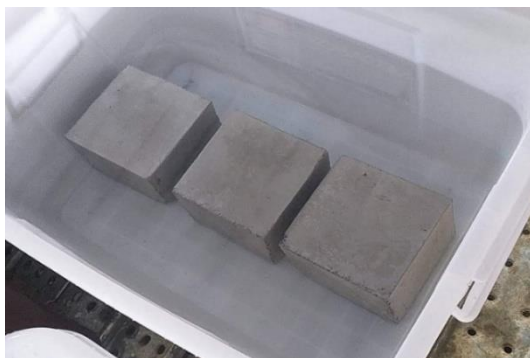
Fig. 5 Concrete cube samples cured in potable water in a normal room condition
