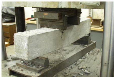
Fig. 11 Flexural test on beam
