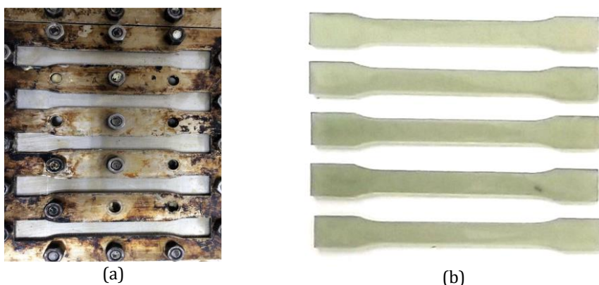
Fig. 2 a) Steel mold b) Test specimens
