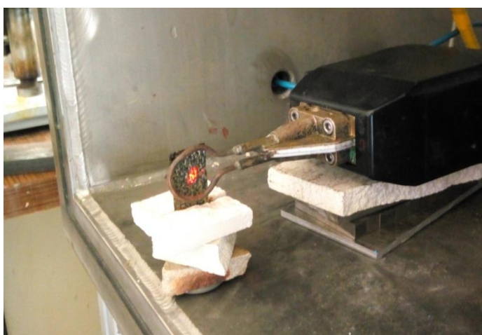
Fig. 1 The cylindrical single turn induction coil.
