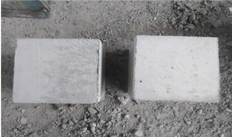
Fig. 5 Surface of Demoulded Cubic Specimens
