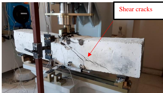
Fig. 3 Shear failures of RC beam
