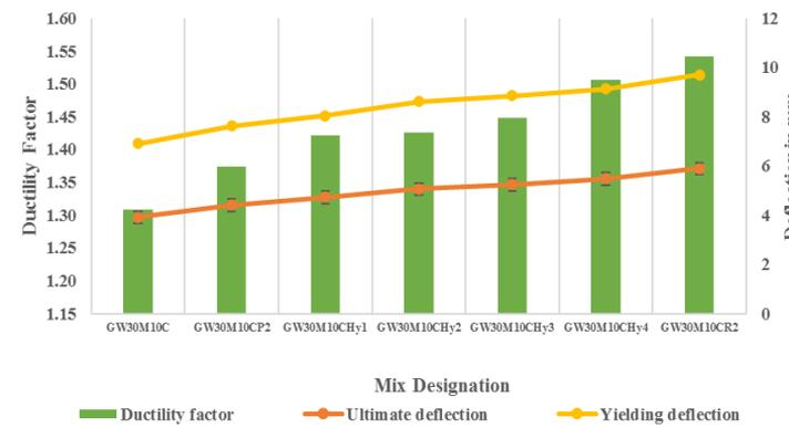
Fig. 4 Ductility factor for various hybrid fibre proportions
