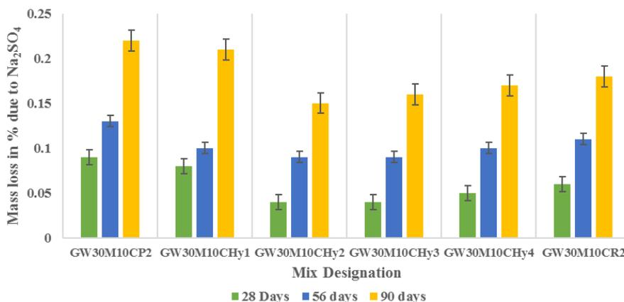
Fig. 11 Mass loss percentage of various HFRGPC specimens under Na<sub>2</sub>SO<sub>4</sub>
