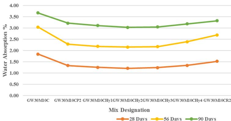
Fig. 6 Water absorption of various HFRGPC specimens
