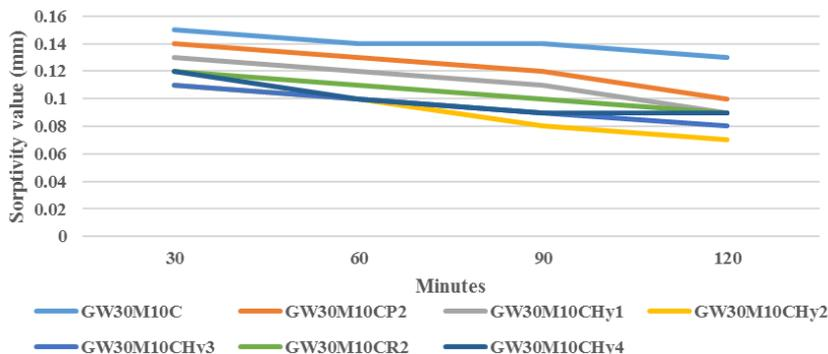
Fig. 7 Sorptivity value of various HFRGPC specimens
