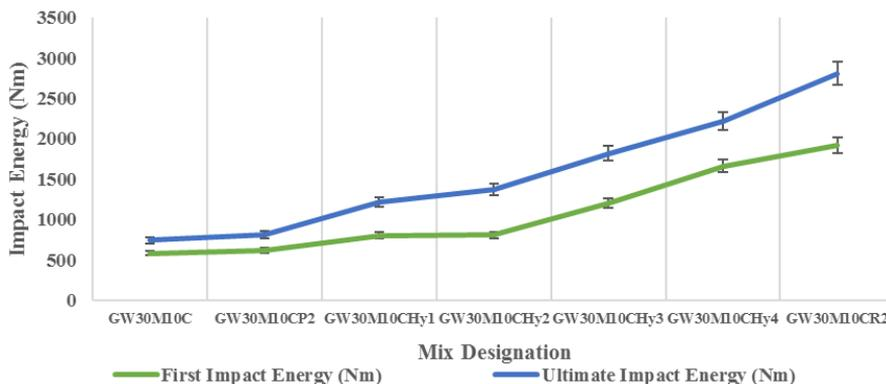
Fig. 5 Impact strength for various hybrid fibre proportions
