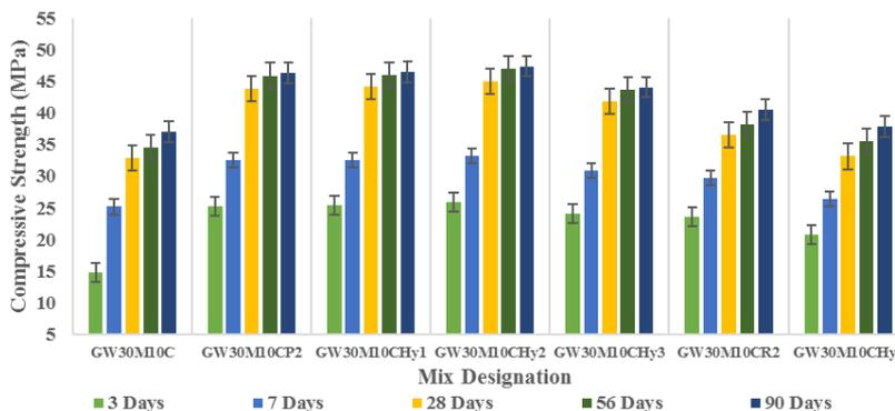
Fig. 1 Compressive strength test results of various hybrid proportions
