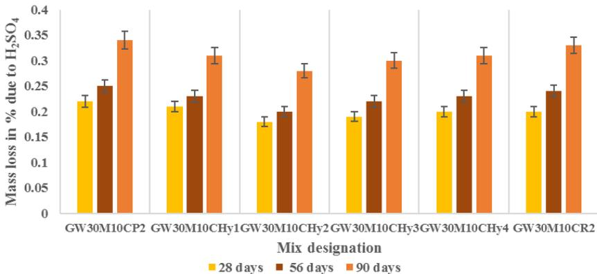
Fig. 10 Mass loss percentage of various HFRGPC specimens under H<sub>2</sub>SO<sub>4</sub>
