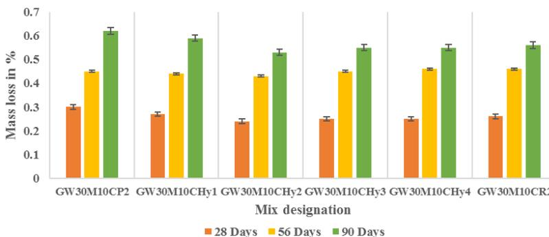
Fig. 12 Mass loss percentage of various HFRGPC specimens under Na<sub>2</sub>SO<sub>4</sub>
