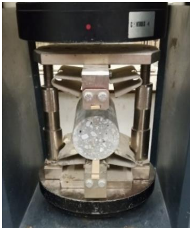
Fig. 3 Test set-up for split tensile strength
