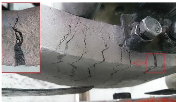
Fig. 5 Fiber bridging in the 28-day L30 S40 Z3-PP specimen at rupture
