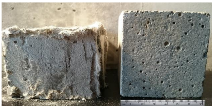
Fig. 1 ECC high ability to withstand compression
