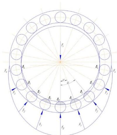
Fig. 1 Scheme of forces distribution on the bearing
